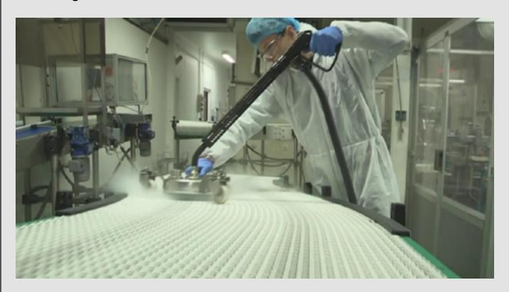
The application of saturated steam makes it possible to clean many different surfaces in the industrial and commercial sector. Industries that requires an effective cleaning and sanitizing. All at low operational cost with a focus on environmental friendly solutions
